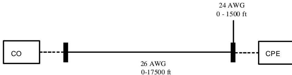
**Figure 12: Bridged Tap Loop Configuration**
